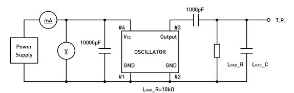
LOAD\_C=10pF (Include Jig stray capacitance)
